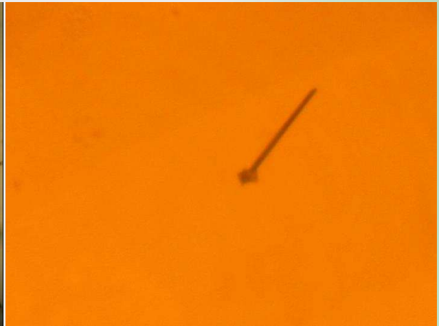
Figure 5: A single spicule was present near the pavilion of the sapphire. Identification by standard techniques could be difficult if the stone was cut with this inclusion alone. Photomicrograph by C. Golecha, magnified 30x.
