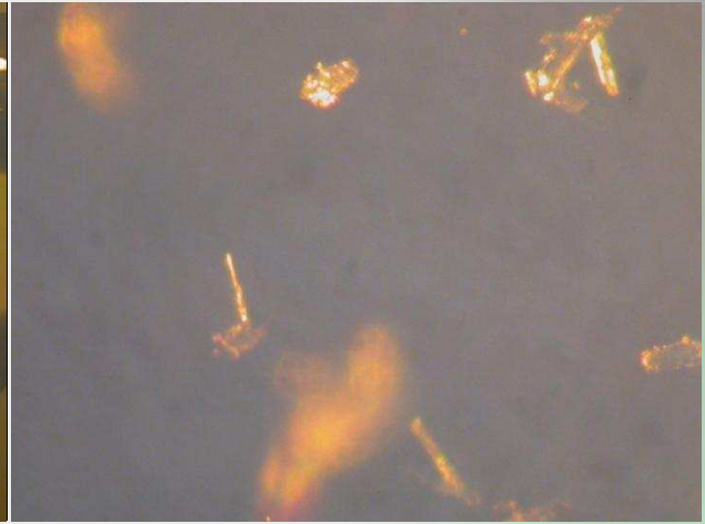
Figure 14: The aggregation patterns of these inclusions in quartz strongly resemble nail-head spicules at certain orientations. Photomicrograph by C. Golecha, magnified 35x
