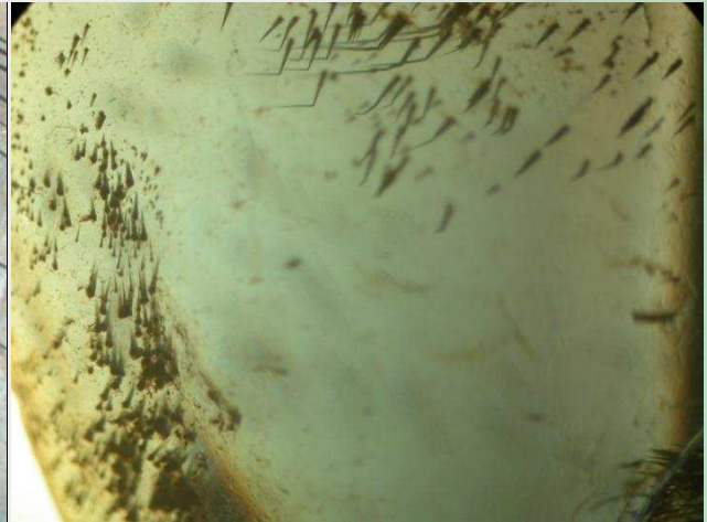
Figure 10: Spicule-like inclusions, some displaying a sharp bend, were observed in various directions pointing toward the interior of the spinel pebble. Photomicrograph by C. Golecha, magnified 30x
