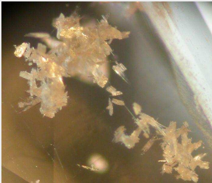
Figure 15: At higher magnification, the inclusions in figure 14 proved to be aggregates of natural mineral, possibly muscovite. Photomicrograph by C. Golecha, magnified 45x
