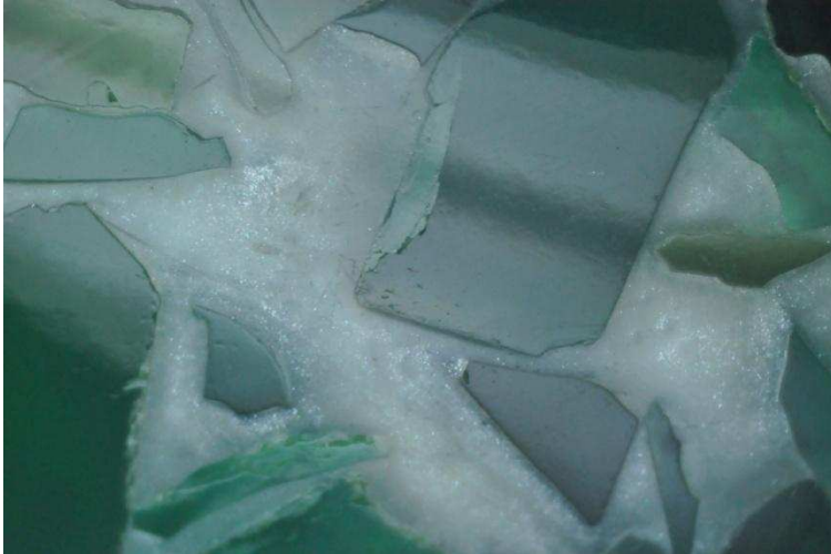
Figure 2: The green and white veined areas distinctly displayed differences in lustre. Note the duller lustre of the polymer filled areas. Magnified 25x
